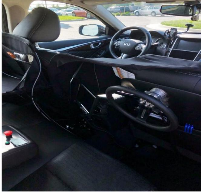
*Figure 9. Redundant steering controls.*
