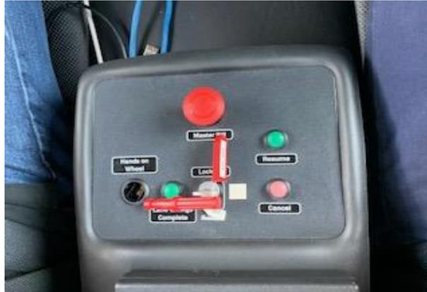
Figure 5. Automation control box.
