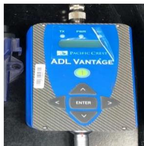
*Figure 4. In-vehicle DGPS unit.*
